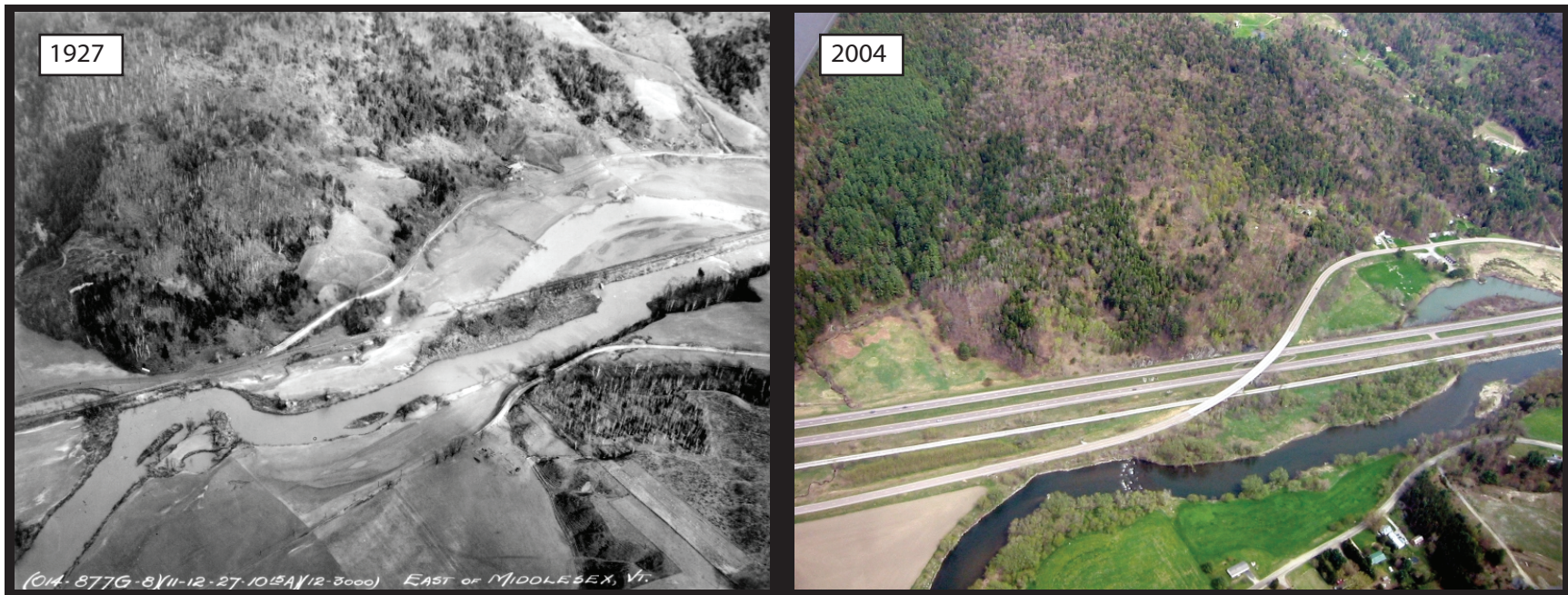
Figure 4. The above photographs are an example of oblique aerial rephotography (University of Vermont, 2012). The image to the left is a 1927 photo of Middlesex, VT. The image to the right was taken 77 years later. In the more recent image, it is apparent that the interstate and state two lane highway have been constructed adjacent the already present railroad, greatly increased the necessary right of way. These images were sourced from the Landscape Change Program database (LS01472_000/ LS01472_001).
